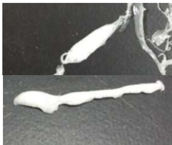
Fig. 5 ABS resin paste ejected through nozzle
