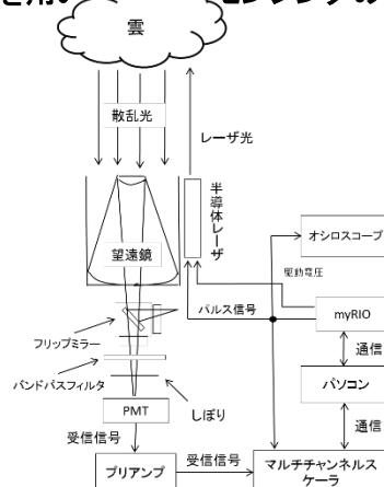
図1 Lidar system (monostatic)
